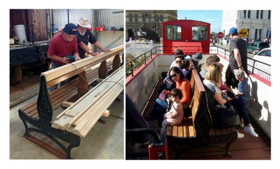
The seat was based on cast metal ends matched to wooden formers and then overlaid with clear pine strips that were formed, stained, varnished and attached with brass screws. The visual effect adds to the experience of traveling on the train and their finish reflects the quality of craftsmanship that was employed in their construction.
