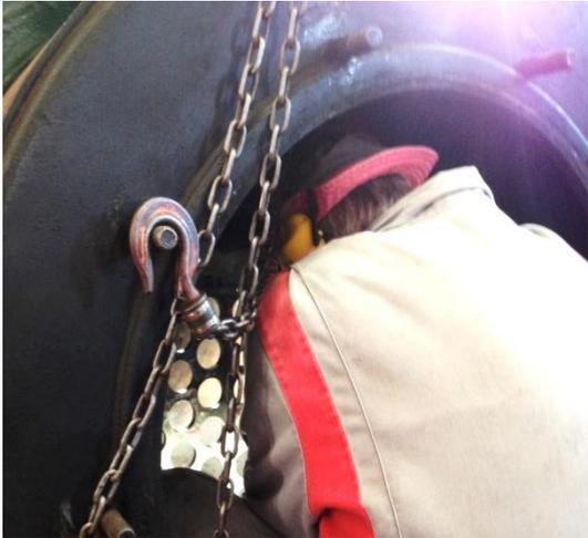
**Steam loco B10's** front tube plate continues to receive attention prior to refitting her boiler tubes. A pressure vessel certified welder has repaired four small imperfections in the plate surface. These welds have since been machined flat and the four adjacent holes re-machined to ensure a snug fit for the tubes. It is hoped that the loco will be running again before the summer season.
