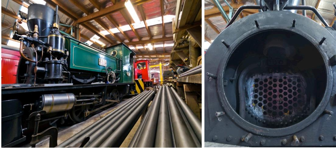
In the next step, the tubes have been cut to the correct lengths – again, an exacting task, because once fitted, both ends of the tube need to be flared out to make a snug fit into the tubeplate holes. They can't be too short or the tubes won't hold in place, and they can't hang out beyond the tubeplate.
