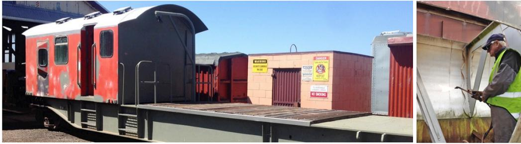
**CW57**, our new track maintenance wagon, was originally built in the 1960s by West Australian Government Railways as hopper wagon XBC 21005. These wagons were built to haul Bauxite ore - the world's main source of aluminium.
