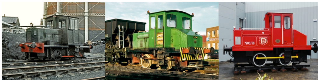
English Huskies – note the buffers and ‘stepped’ cab mount. Pictures courtesy Gordon Edgar
