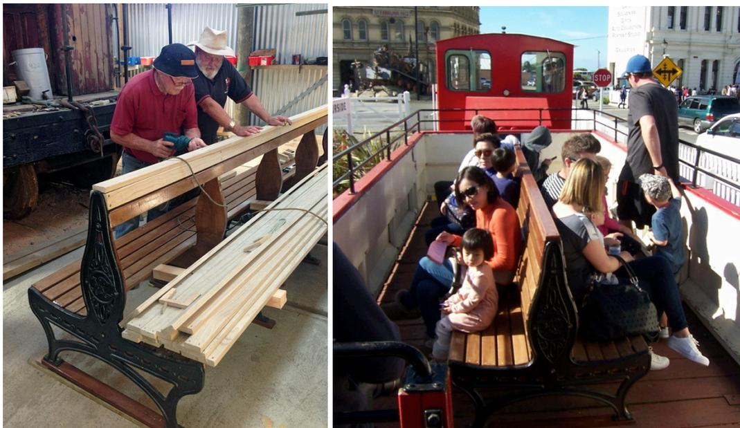
The seat was based on cast metal ends matched to wooden formers and then overlaid with clear pine strips that were formed, stained, varnished and attached with brass screws. The visual effect adds to the experience of traveling on the train and their finish reflects the quality of craftsmanship that was employed in their construction.
